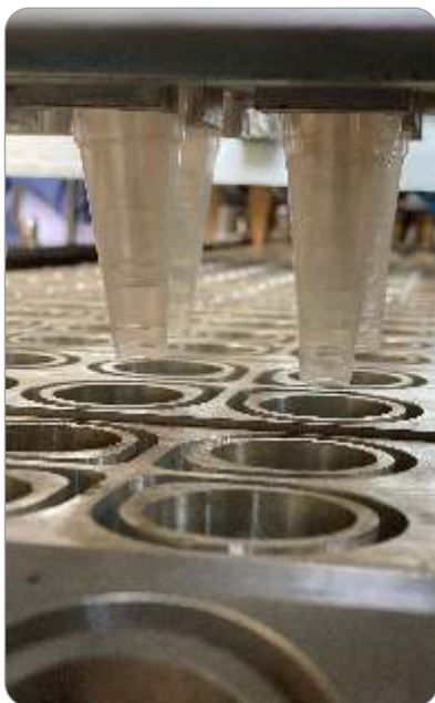
Thermoformed Cups Dispensing Station
